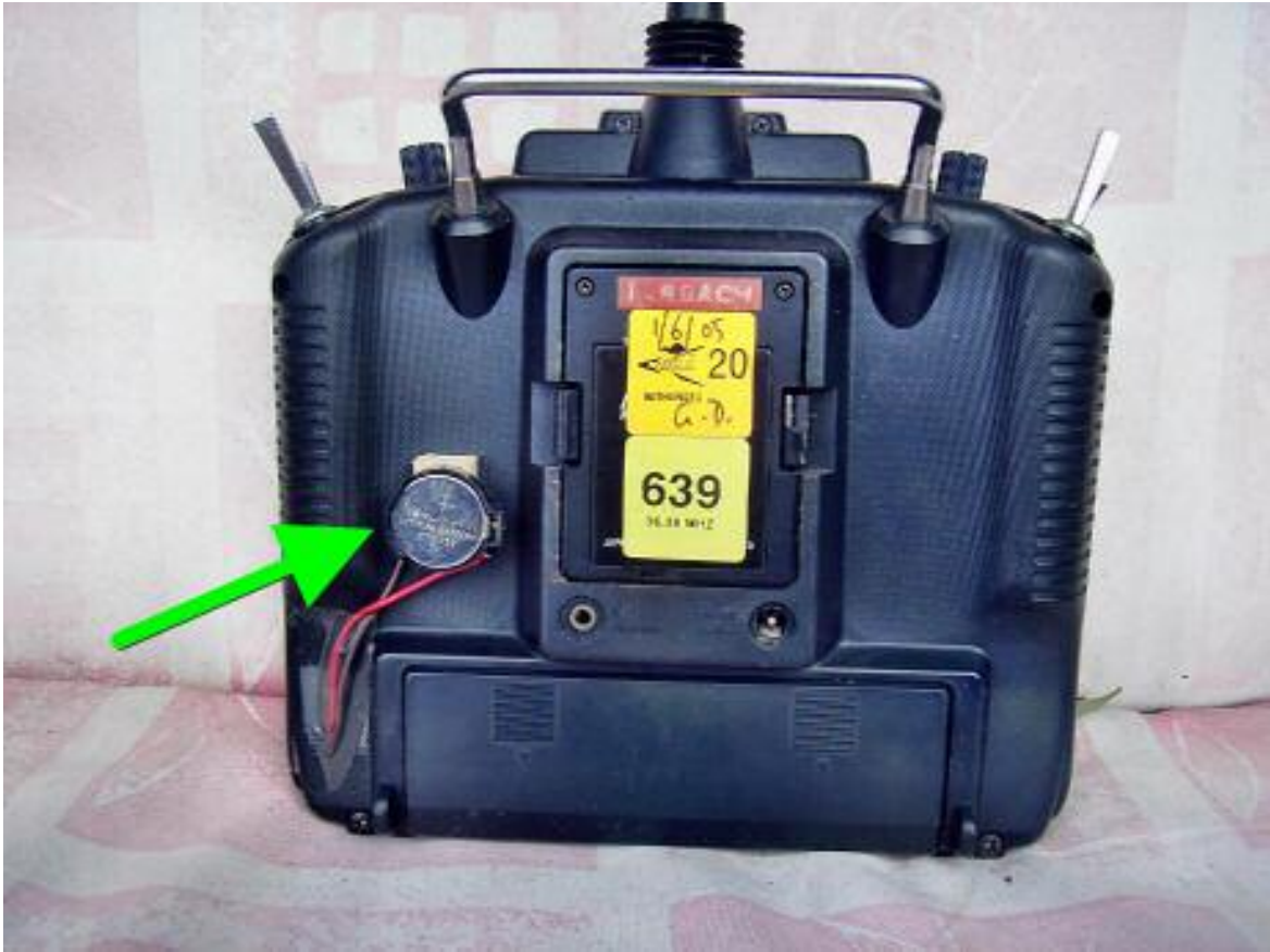
View of the JR388 with the CR2032 lithium backup battery mounted externally in a button style battery holder on the back of the transmitter case.
