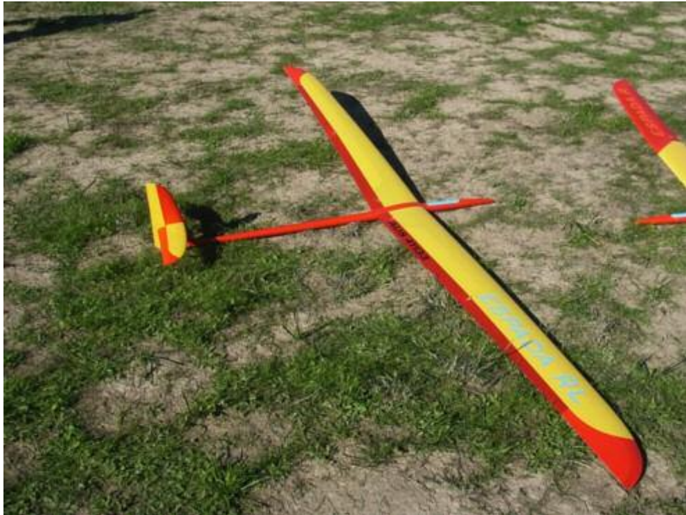
This is one of several examples of the Espada RL seen at Jerilderie this year. Despite having a wingspan of about 3.7 metres it weighs less than 2 kg.
