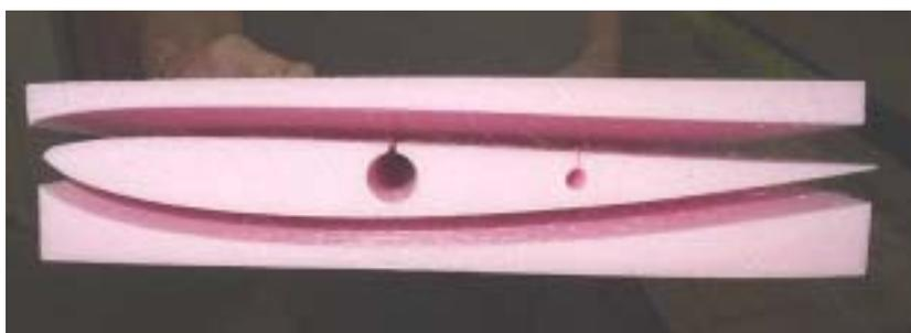
*This core is cut from extruded polystyrene and shows the tube spar hole and wiring hole cut in. All is explained in the DVD.*
