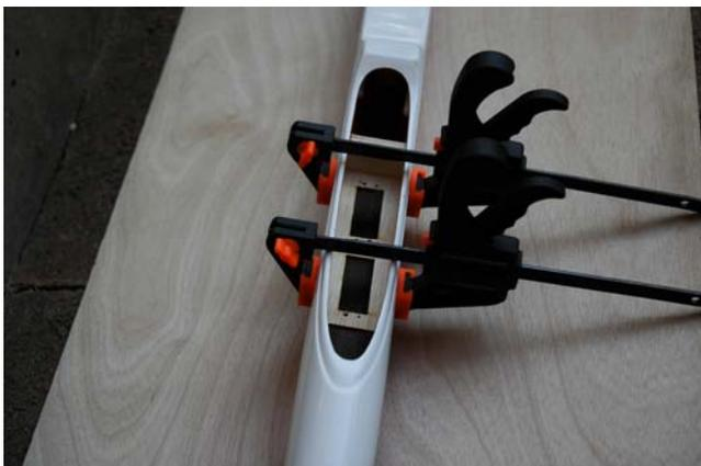
Next, I marked the outer sheaths of the pushrods, and cut them to size. I rolled a length of 13mm wide masking tape around the diameter of the outers, every 120mm or so, down their length. A dab of epoxy on each masking tape collar, soon had them attached to the inside of the fuselage. They need to be anchored, to prevent any flexing. Make sure you get a smooth run, as you don't want the inner rods to bind. Test fit the inners, making sure that the ball link collars go far
