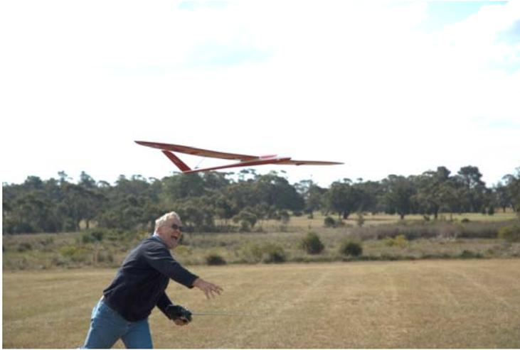
It went up at a 70-degree angle, straight as an arrow, and showed no signs of stalling. There was no need for rudder during the launch, and a shallow dive and zoom, for a ping off, saw an additional 10m or so in height gain. The plan for the first flight was to get used to the flying characteristics, check aileron, rudder and elevator response, and also to see what it did on application of flaps. The Starling was set up on my JR 9X11, so I had all of the mixing capabilities I would
