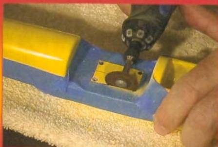
Shows a Dremel tool being used to cut out the servo bay on a fiberglass fuselage.
