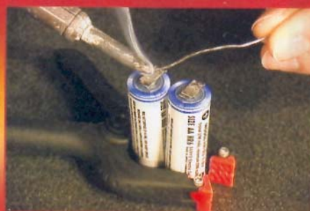
A section of the DVD shows how to solder battery packs.
